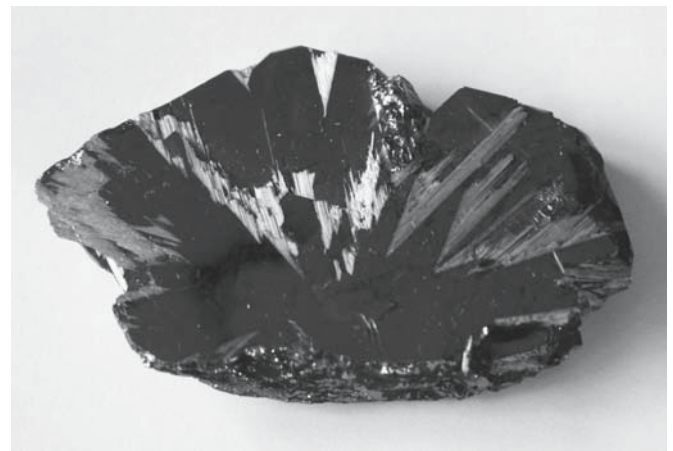
FIGURE 36.30 Rutile growing in hematite. This combination often causes patterns in quartz crystals.
