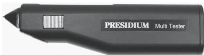
FIGURE 36.18 Pocket-sized instrument for measuring thermal conductivity.
