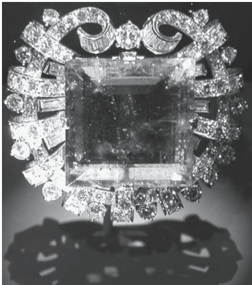
FIGURE 36.21 An emerald cut in the classical style that minimizes the likelihood of fracture.
